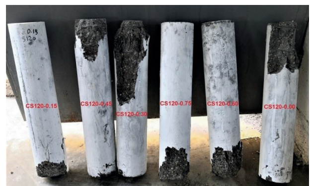
Fig. 8 Failure patterns of short columns
