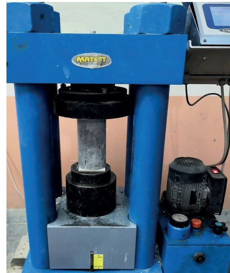
Fig. 5 Testing of control specimens for compressive strength
