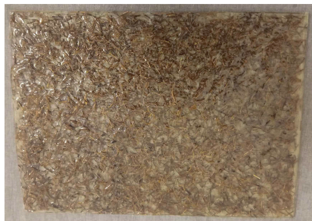
Fig. 1 Date palm fiber and epoxy resin plate
