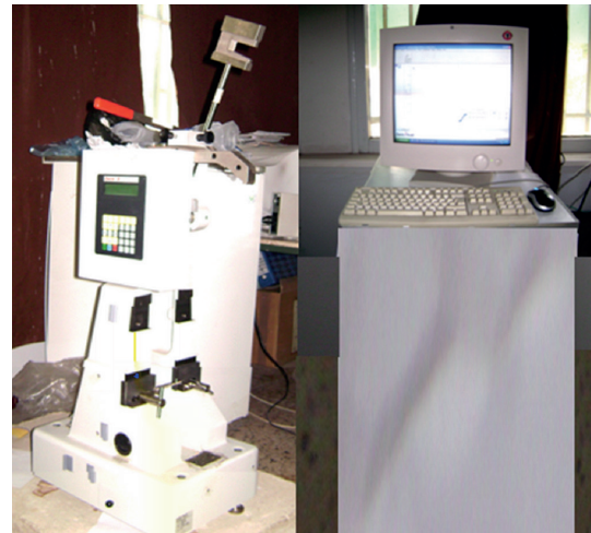
Fig. 3 Zwick/Roell type Charpy impact machine used
