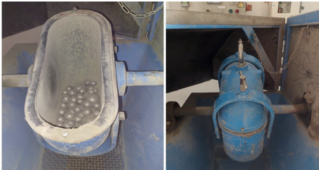
Fig. 1 Grinding of brick waste
