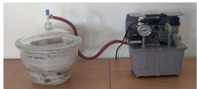
Fig. 6 Test of Spreading Consistency (a) and experiment on air absorption (b)
