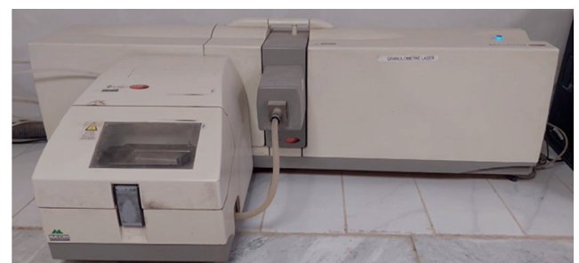
Fig. 2 Laser diffraction analyzer
