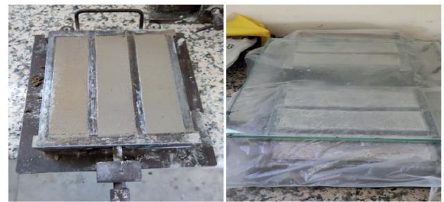
Fig. 5 Storage of specimens
