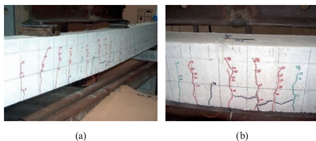
Fig. 10 Crack distribution at beam B-G3 (bypassing 20Ø): (a) general view, (b) detail view
